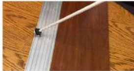
STAIR MOCK UPS SHOWED THAT STANDARD NOSING WOULD CAUSE DANE TIPS TO OUCH
